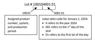
For traceability purposes, NuTek can determine the plant location, production line, and the date of manufacturing of the product from the lot number
